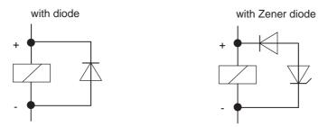
Figure A-9 Circuit for coils operated with DC voltage
